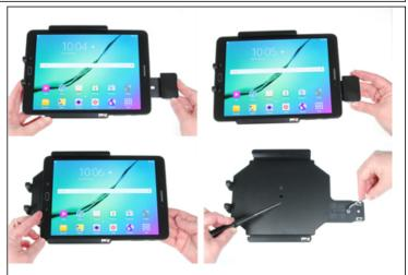
2. Remove the spring block carefully, keeping the adjustable arm exactly in position. Remove the device carefully, making sure the side arms stay exactly in position. Fix the size of the holder by tightening the screws on front of the holder as well as the screw on the adjustable arm.
