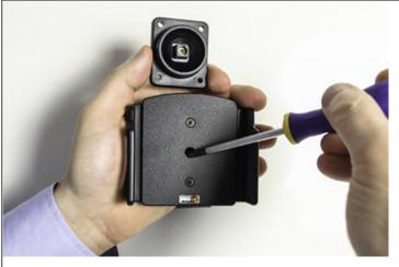
2. To install the holder onto a mount: Completely loosen ONLY the one screw in the center of the holder. (the screw will not come out and may feel like it is just spinning) Then, using light force, pull the swivel base plate away from the back of the holder. This will separate the Device Holder portion from the Tilt-Swivel base plate.
