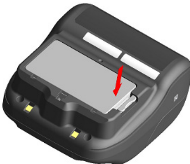
Figure 8-3 Installing Battery Pack (2)
