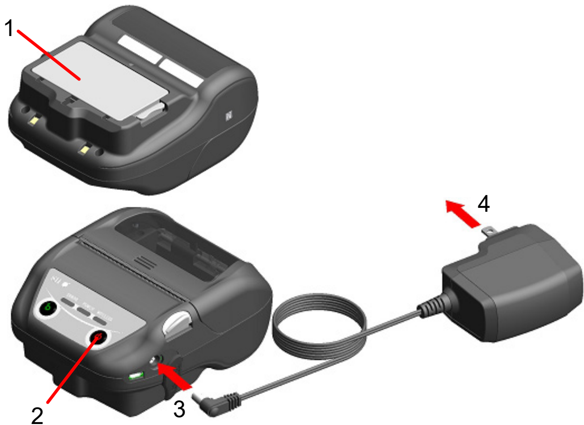
Figure 14-1 Charging in Power On Charging Mode by AC Adapter
