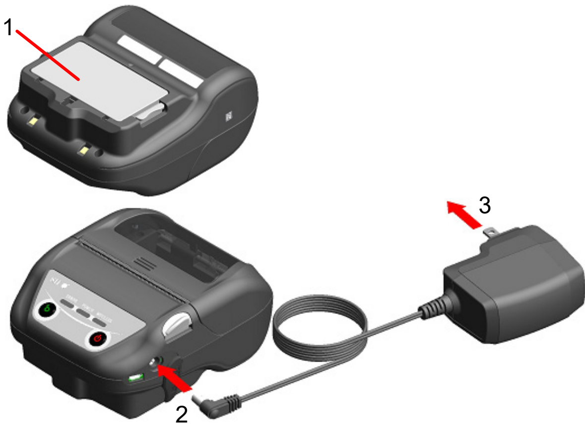
Figure 14-2 Charging in Power Off Charging Mode by AC adapter
