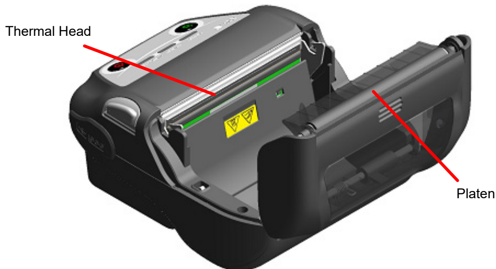
Figure 18-1 Cleaning Thermal Head / Platen
