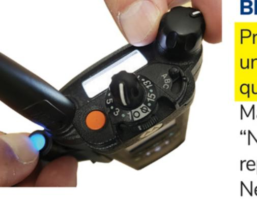
radio, press down on the clear PTT button on the BT Adapter & turn the radio on at the same time. When BT Adapter is flashing Blue/Red release. When both BT Adapter & Nighthawk are solid Blue for a moment both units are paired. No need to repeat the pairing process when this is achieved.
