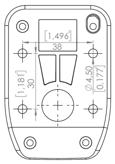
Image in 1:1 size. Can be used as an drilling template.
