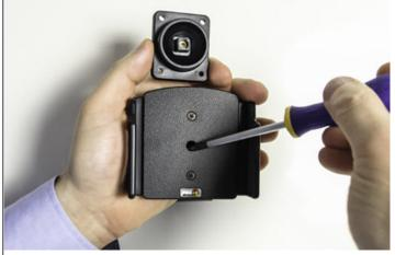
2. To install the holder onto a mount: Completely loosen ONLY the one screw in the center of the holder. (the screw will not come out and may feel like it is just spinning) Then, using light force, pull the swivel base plate away from the back of the holder. This will separate the Device Holder portion from the Tilt-Swivel base plate.
