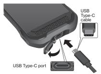
When charging is complete, remove the cable from the port and securely close the cover.
